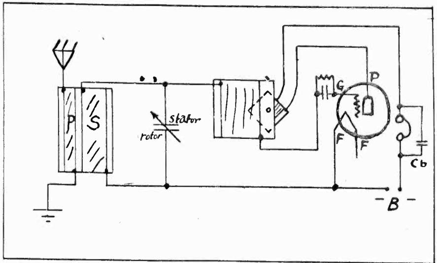
Fig. 4. Mounting and Hook-up of Split Secondary
