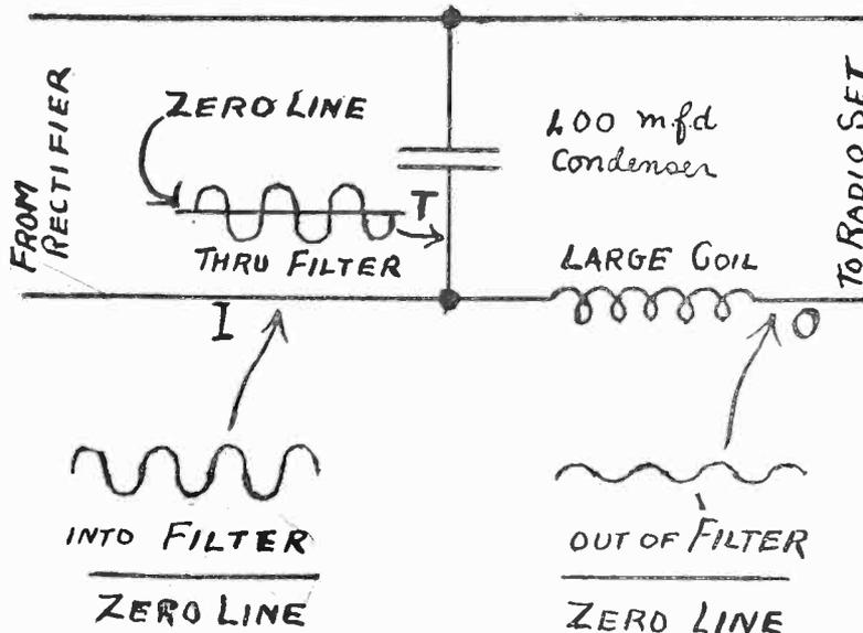
Fig. 7. Current In and Out of Filter
