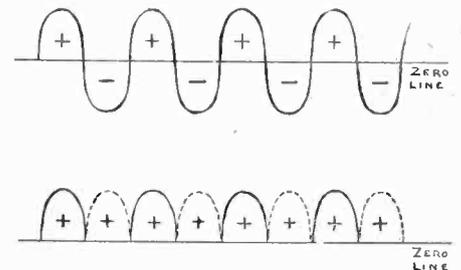
Fig. 5. Current from Rectifier
